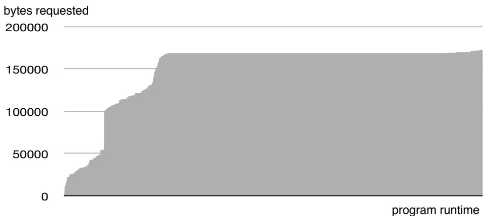
Figure 6.7: Runtime distribution of bytes requested from the server for the Floating-PointCheck benchmark for SpecJVM.
